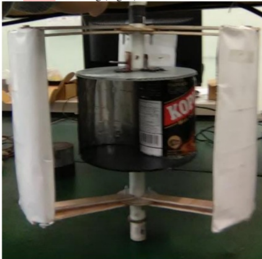
Fig. 3. Hybrid wind turbine (Savonius - Darrieus)
