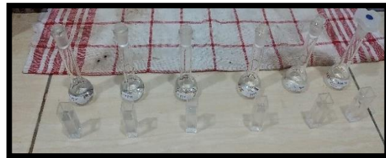
Gambar Lampiran 8. Deret standar asam tanat 0,5 ppm, 1 ppm, 2 ppm, 4 ppm, 8 ppm
