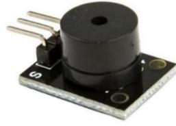
**Gambar 2.16** Modul *Buzzer* 5V KY-012
