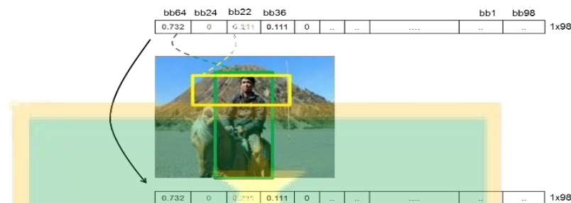
Gambar 2. 17 Tata letak (grid) algoritma yolo hasil perbandingan false bounding box 22 (Hidayatulloh, 2021)
