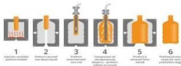
Gambar 2.6 Proses Stretch Blow Mold
