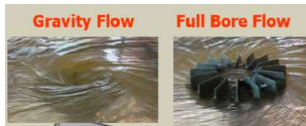
Gambar 19. Aliran gravity flow dan full bore flow
