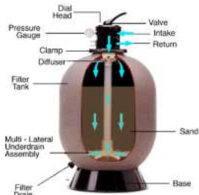
Gambar 5 Sand Filter Tank
