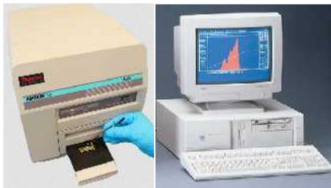
Gambar 3.3 TLD Reader Harshaw Model 3500
