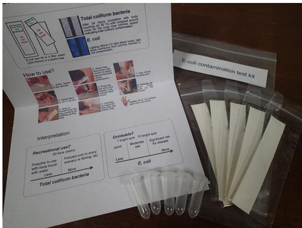
Fig. 3. A potential device designed. Manual, alcohol in microtube, and E. coli test strips are packed in a plastic bag.
