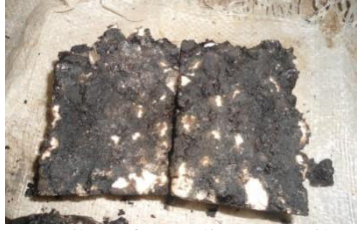
Figure 13. Briket after Indirect Tensile Strength Test
