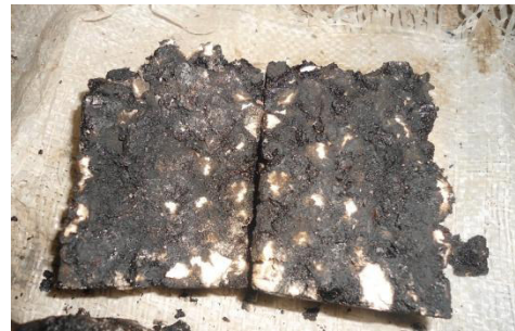
Figure 11. Briket after Indirect Tensile Strength Test
