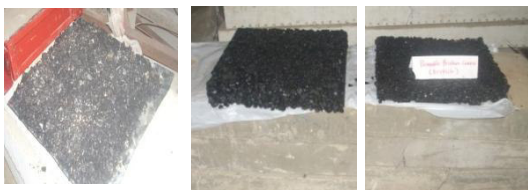
(a) (b) (c) Figure 7. Permeable asphalt pavement
