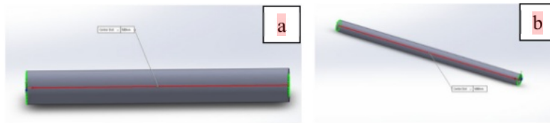
FIGURE 7. Two different lengths for straight pipe exhaust part (a) 500 mm to (b) 1,000 mm respectively
