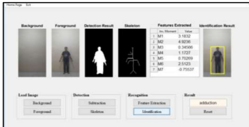
Figure 10 Identification process and the identification the Range of Motion
