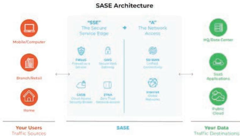
**Gambar 5.20.** Secure Access Service Edge (SASE)
